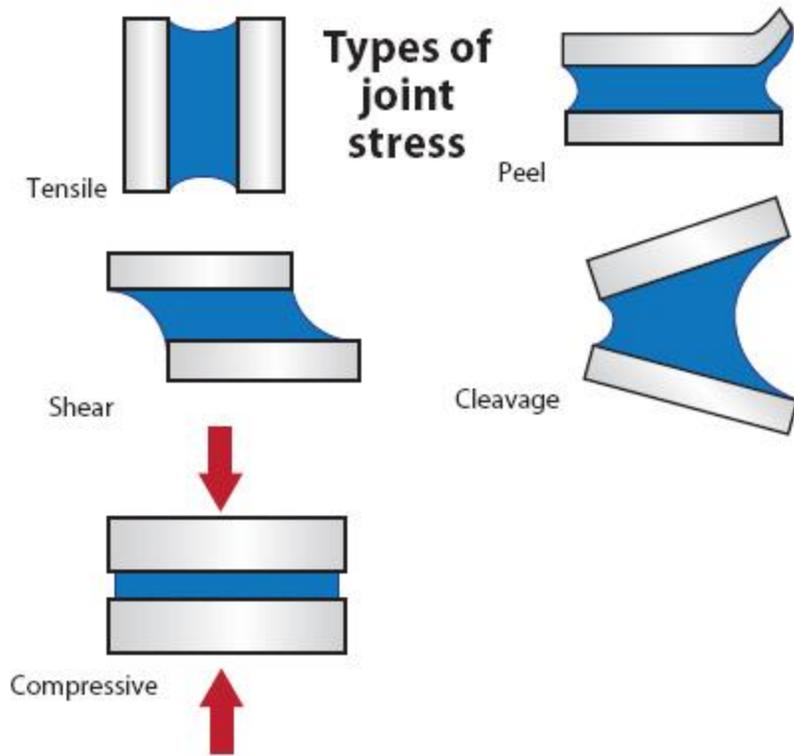
Adhesive Stress Failure Points
