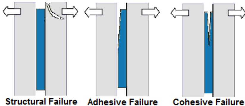
Three Types of Adhesive Failure
